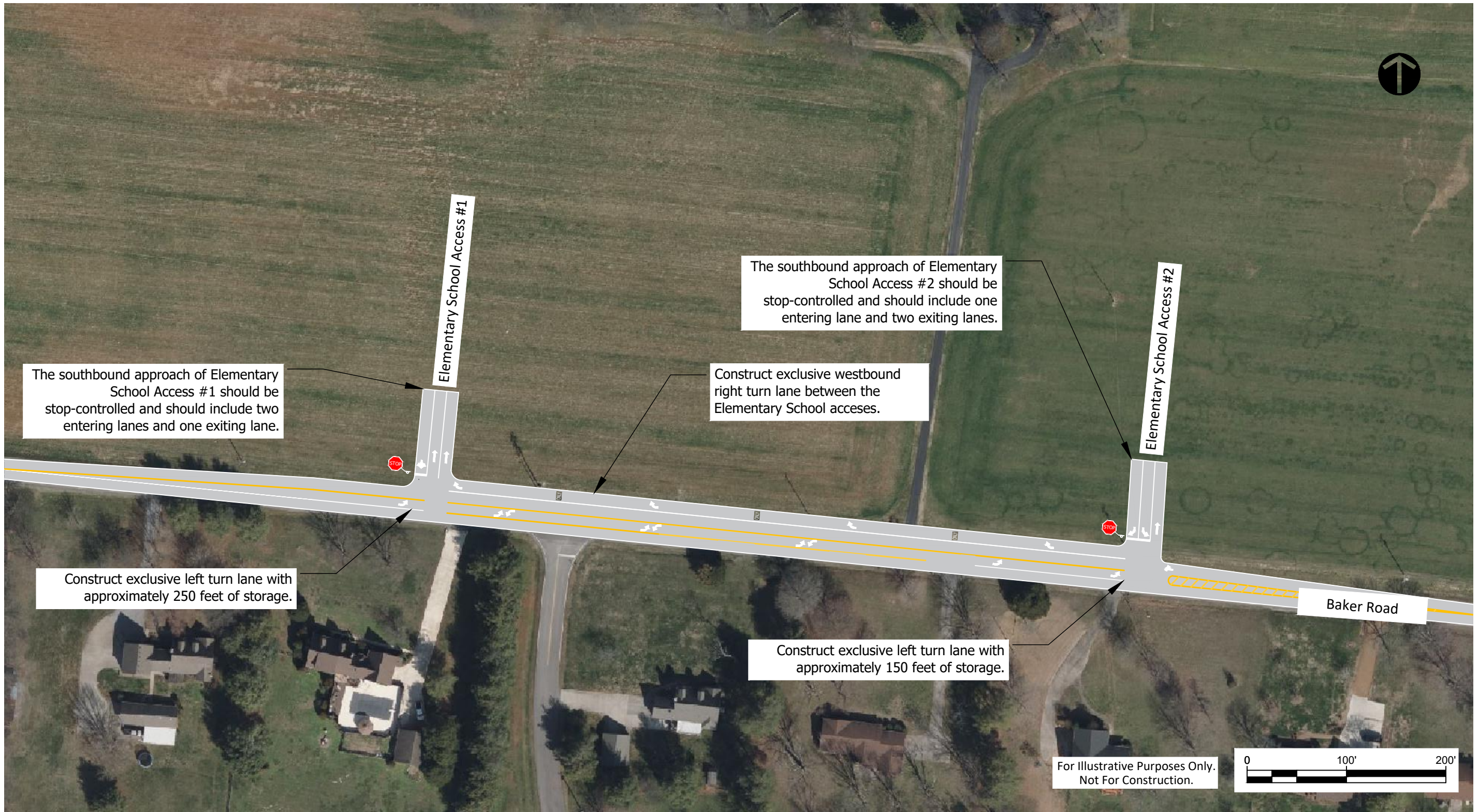
Figure 11: Recommended Short-Term Improvements along Baker Road
